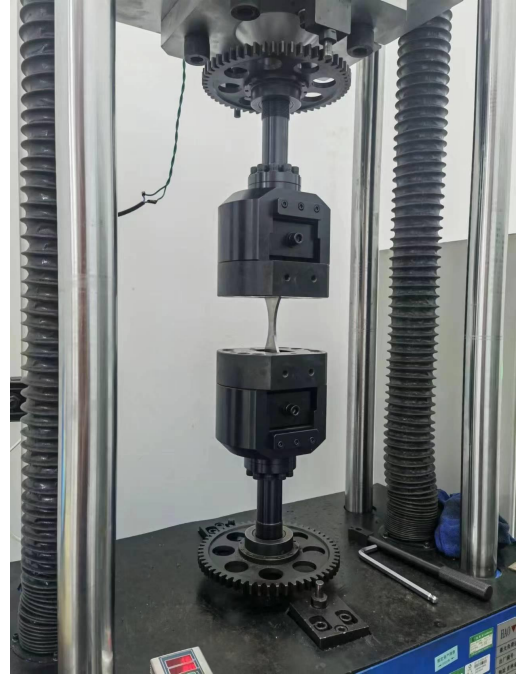
Patented new automatic centring fatigue fixture
