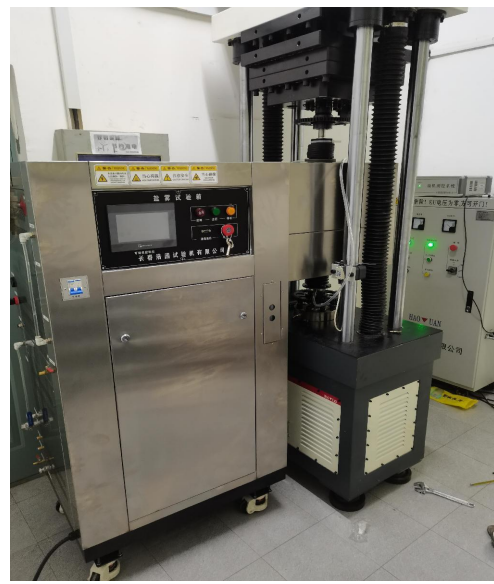
High temperature atmosphere furnace and high temperature fixture
