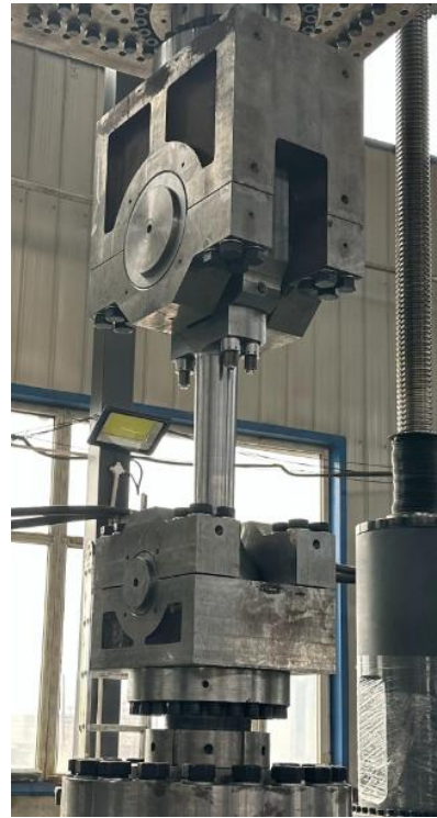
3000kn large tonnage engine connecting rod fixture
