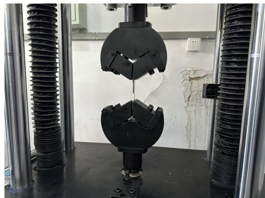
Patented new automatic centring fatigue fixture
