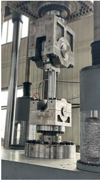
3000kn large tonnage engine connecting rod fixture
