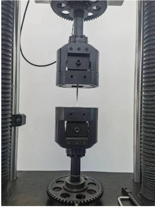
Patented new automatic centring fatigue fixture
